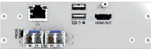
R488-BIPSR - Fiber with redundant link interface
